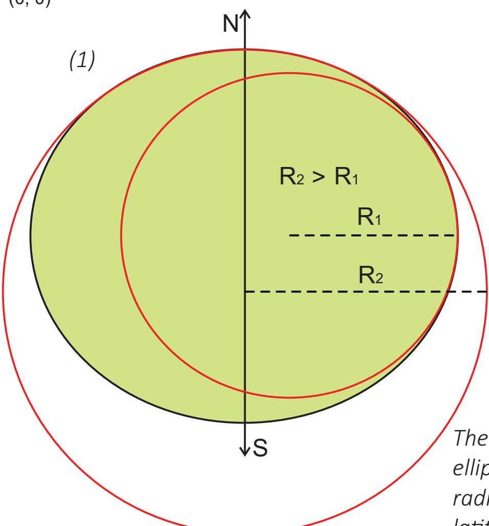
The curvature of the ball adapts to the surface of the ellipsoid, therefore the radius  $R$  is variable (1). The average radius  $R = 6371$  km is best adapted for a 35 degree N or S latitude (2). Both options are included in the programme.
